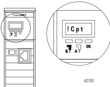
To update the keeper signature, perform this procedure when a secondary chassis will not synchronize and its CNB modules show !CPT.
