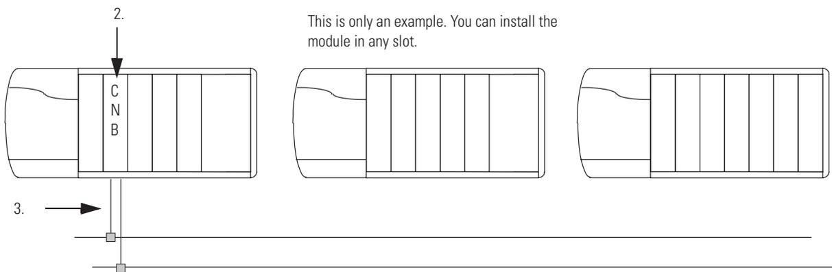
2. Install a 1756-CNB/D/E or 1756-CNBR/D/E module. See ControlLogix ControlNet Bridge Installation Instructions, publication 1756-IN571.
