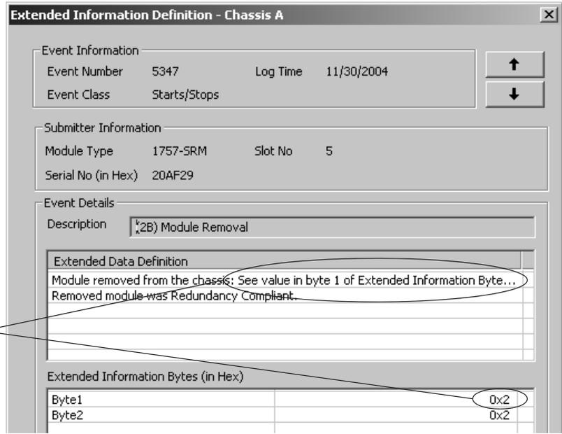
Someone removed the module for slot 2. Or the module failed.
